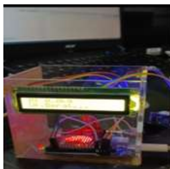
Gambar 3. Pendeteksi Stunting Berbasis Arduino Uno
